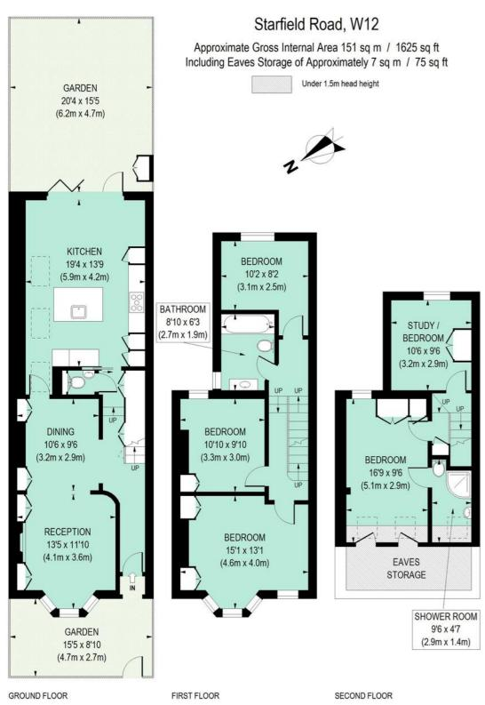
Floor Plan produced for Philip Wooller by Mays Floorplans ⊚ . Tel 020 3397 4594 Illustration for identification purposes only, not to scale All measurements are maximum, and include wardrobes and window bays where applicable
